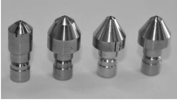
Fig 1: An example of a Rockwell diamond indenter from each of the 4 suppliers
